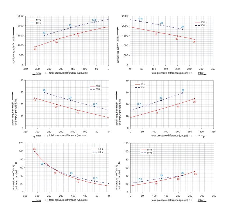
The performance curves are based on air at a temperature of 15 °C and an atmospheric pressure of 1013 mbar with a tolerance of +/- 10 %. The total pressure differences are valid for suction and ambient temperatures
